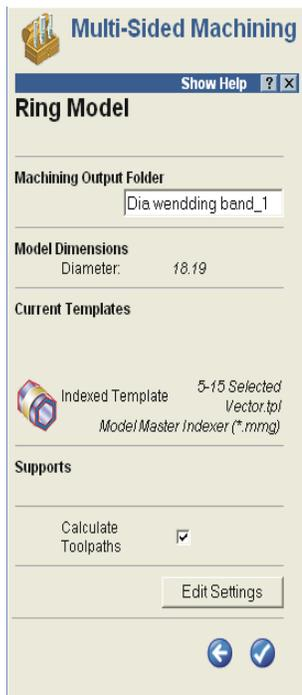
Pick Ring and click next on the arrow key the diameter should be about the size of the ring and 40 pix resolution is good. The next window is machining orientations. Pick inside.
