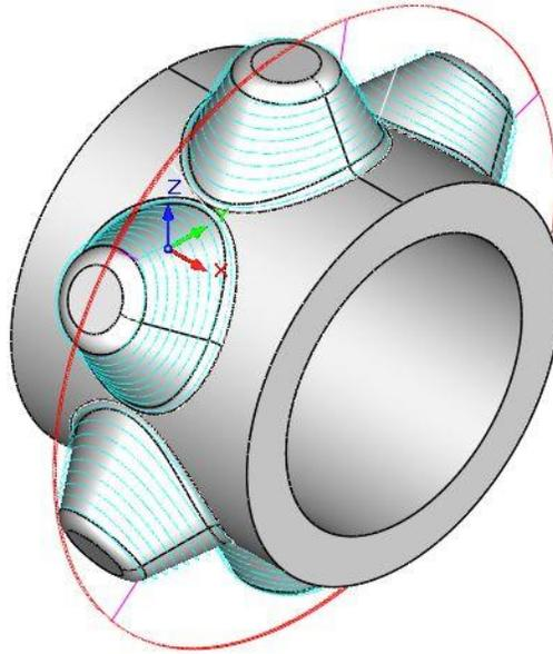
29. **Projection Pocketing Method \*\*** - similar to 3 Axis Projection Pocketing and is used for pre-finishing and finishing of pockets with sculpted bottoms and/or sides. The pockets are defined by regions, and successive inner offsets of these outer regions are generated. The tool moves along these offset curves while following the contours of the part below.
