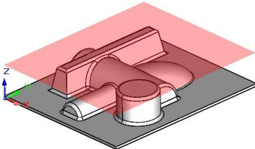
6. **Z level Picking for Horizontal machining methods** – Allows you to pick Z level containment by snapping to a point on the model.
