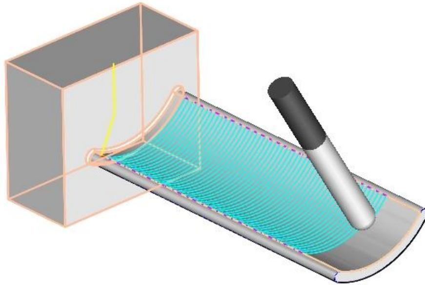
35. **Swarf Machining** \*\*\* - material removal is performed by the sides of the cutter.
