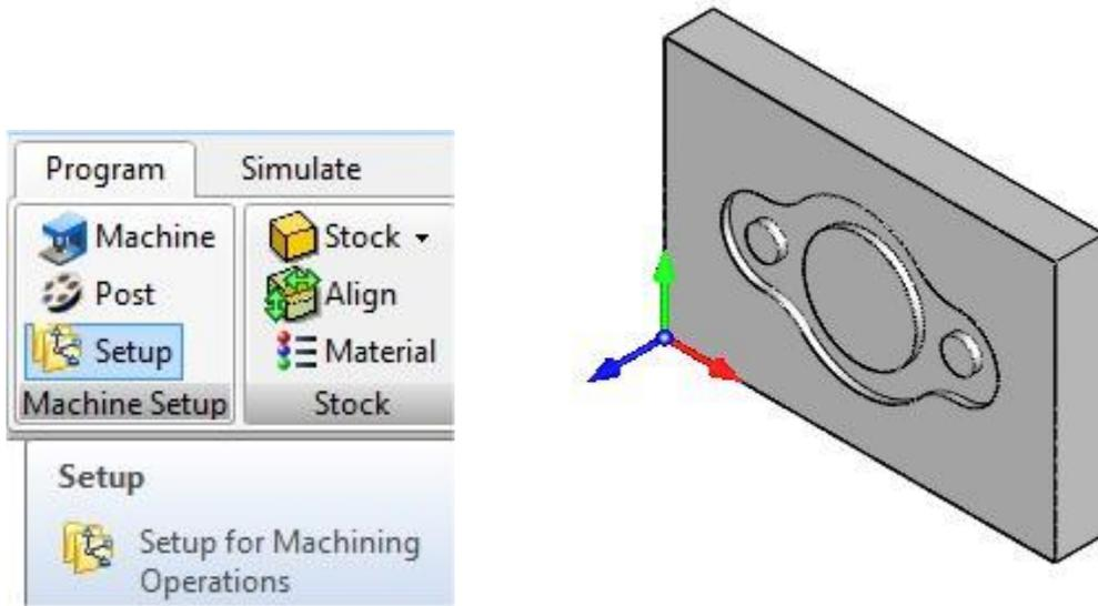
22. **Set Work Zero** - defines the workpiece (part or stock) origin. Work Zero translates the MCS origin from the Setup to the desired location.
