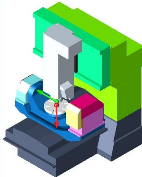
42. **Visualization of machine motions \*** - simulate actual machining of the generated toolpaths with machine tool simulation.
