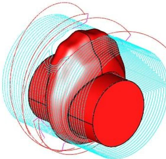
28. **Radial Finishing Method \*\*** - similar to 3 Axis Horizontal Finishing used for pre-finishing or finishing except that the levels in this case are concentric to the axis of rotation
