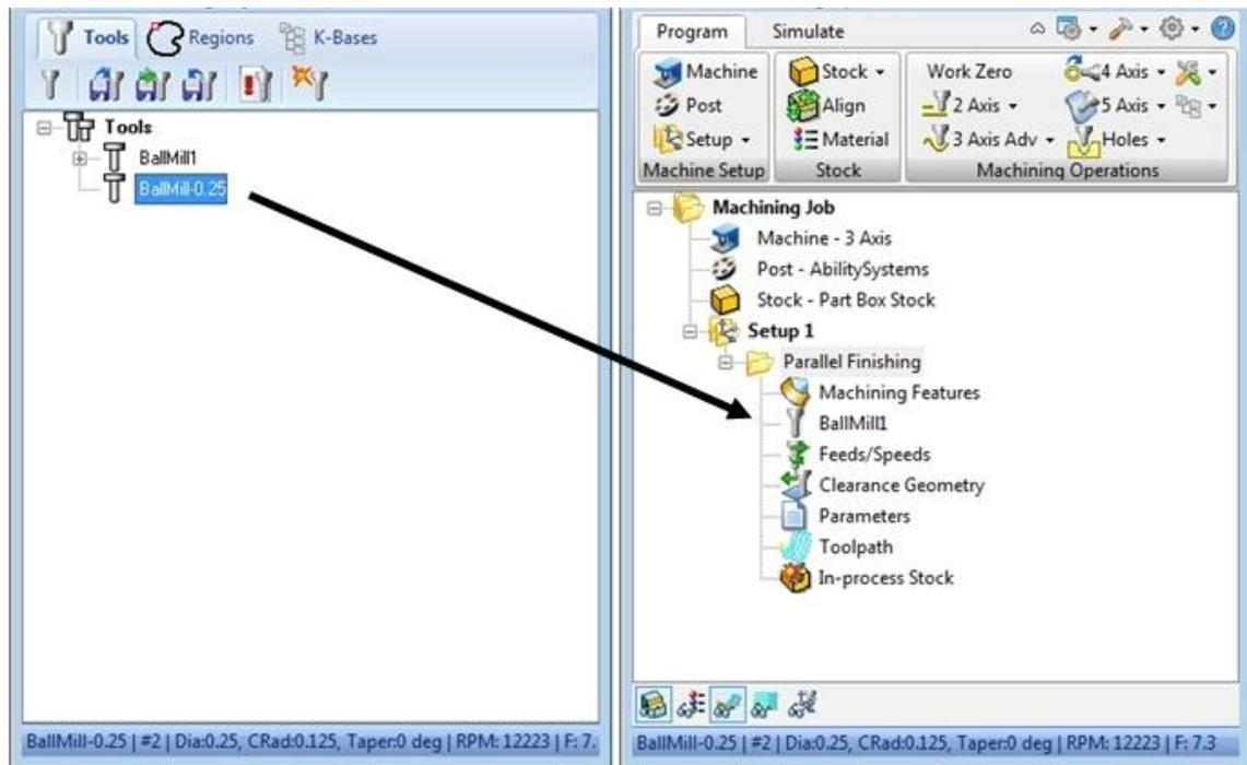
12. **Drag & Drop knowledge base operations to MOPs browser** - This provides the flexibility for the user to select a Setup or an operation under the K-Bases tab and drag it to the Machining Operations browser for programming.
