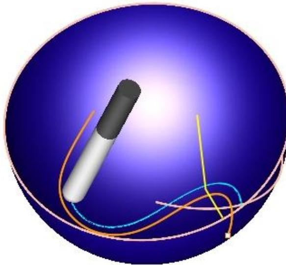
34. **Surface Normal Machining** \*\*\* - similar to parallel finishing where tool moves along a cut pattern, following the contours of the part geometry below and stays normal to the surface
