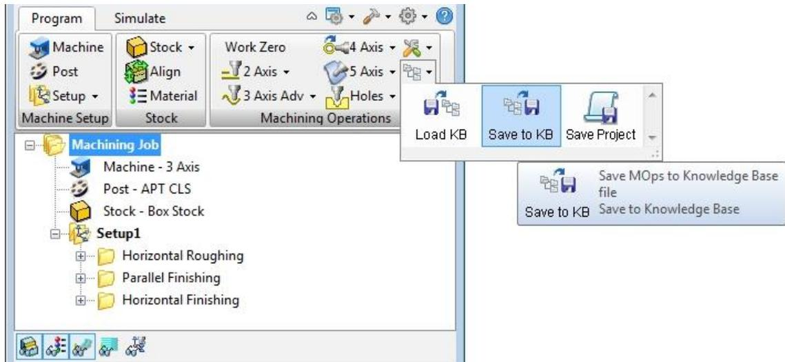
9. **Default Parameter Saving** - Default Knowledge Base allows user to set default parameters for machining operations. This allows the reuse of the machining parameters without having to enter the same parameters when creating new machining operations on same part or new part files.
