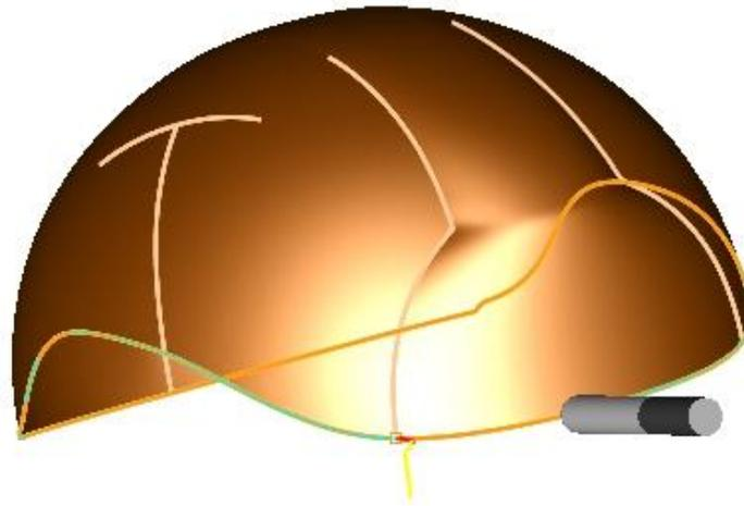
31. **Flow Curve Machining** \*\*\* - toolpath flows on the part surfaces following the curves.
