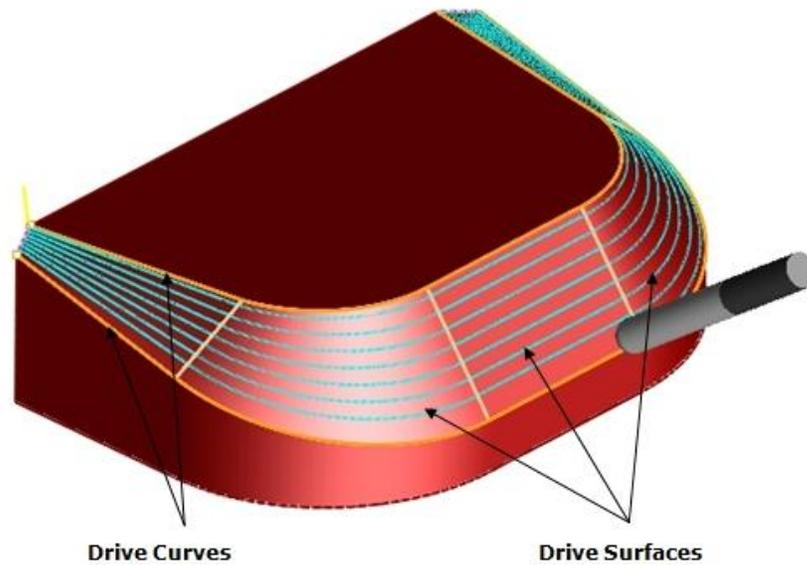
33. **Drive Curve Machining** \*\*\* - used for trimming blow molds and sheet metal dies and the tool follows the curve.
