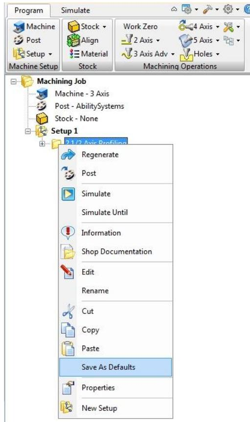
10. **Graphical Toolpath Editor** \* – Perform non associate toolpath edit. Once a machining operation is created, the toolpath can be edited to add post-processor commands.
