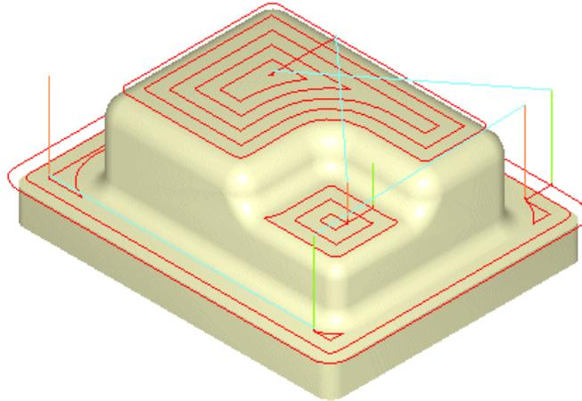
26. **Start Point Definition in Horizontal Roughing** - Allows you to select a point to set the start point for entry motion.
