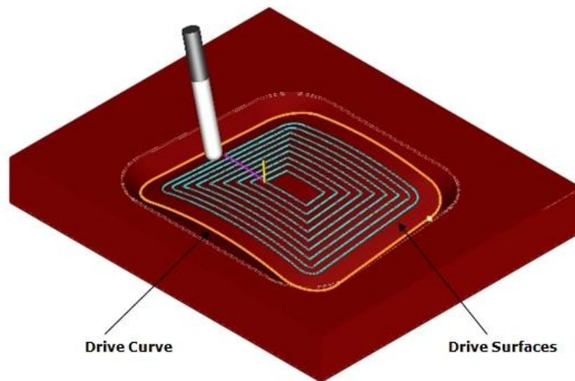
32. **Between 2 Curve Machining** \*\*\* - morphs between two curves. The toolpath makes a gradual transition from one curve to the other and the tool stays normal to the surface.
